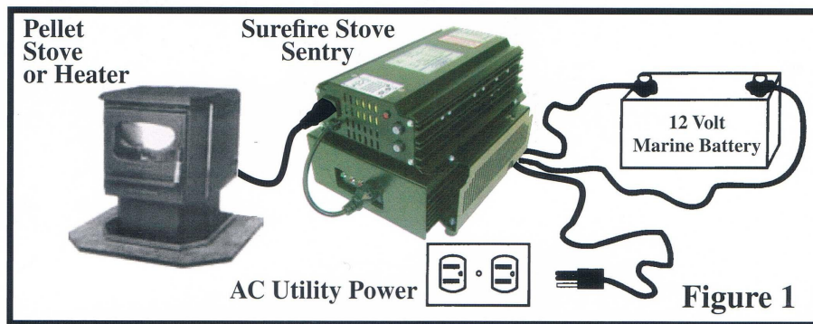
Figure 1 illustrates the interconnection between the pellet stove, Surefire Sentry and battery.
