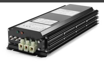
Model 7058 is designed to meet the emerging need to charge lithium 48V battery banks from 24V systems. Model 7058 will output 25A @ 58V in full charge mode and can be operated while load is drawn from the battery bank being charged. Off the shelf units are ideal for use with lithium iron phosphate batteries. Model 7058 is microprocessor controlled and can be programmed at factory for operation with other battery types.
