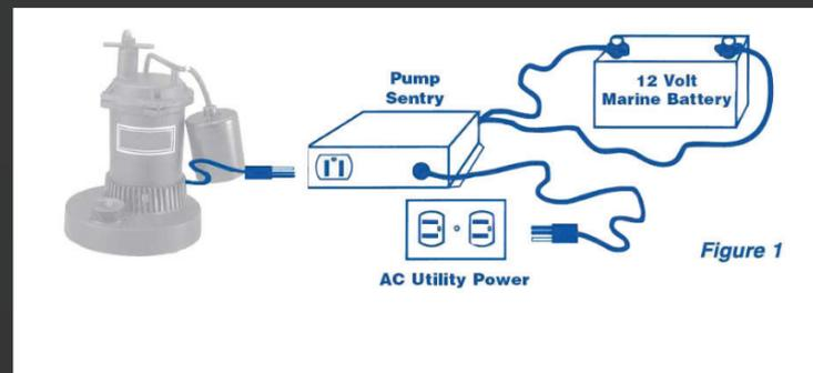
When electricity is present, the Pump Sentry charges a 12-volt battery and monitors the power line. At the instant that a power failure occurs, the Pump Sentry converts the energy stored in the battery to AC power to operate your pump. When AC utility power is restored, the Pump Sentry automatically switches your pump back to AC utility power, recharges the battery, and resumes monitoring the power line.
