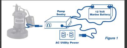
pump back to AC utility power, recharges the battery, and resumes monitoring the power line.
