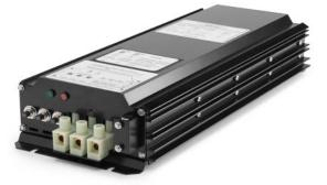
Model 6929 is designed to meet the emerging need to charge lithium battery banks from 12V systems. Model 6929 will output 45A @ 29V in full charge mode and can be operated while load is drawn from the battery bank being charged. Off the shelf units are ideal for use with lithium iron phosphate batteries. Model 6929 is microprocessor controlled and can be programmed at factory for operation with
